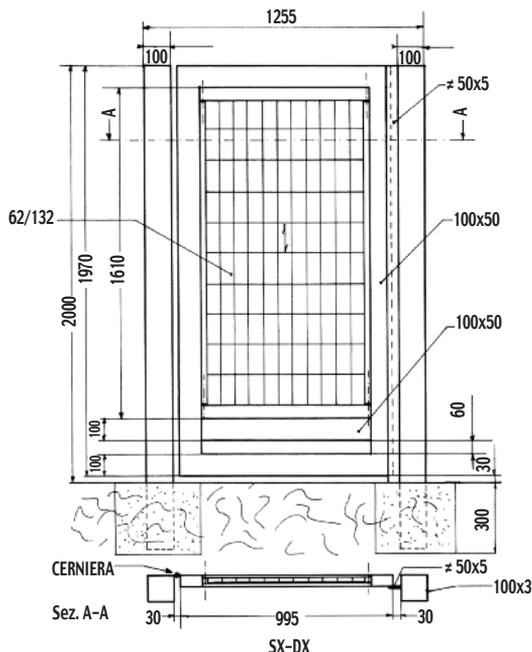
Struttura perimetrale in tubo 100x50x3, base in due tubi 100x50x3, montanti, pilastri in tubo 100x100x3
